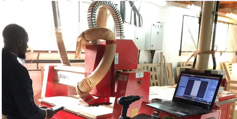
Use of CNC machinery to carve wood for furniture manufacturing
