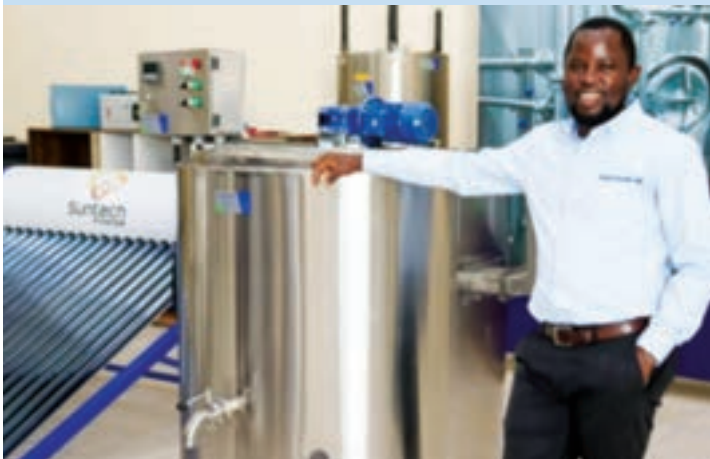
Biogas powered milk pasteurization machine manufactured by Techwin Limited at their workshop in Techwin industrial Park in Nairobi, Industrial Area.
