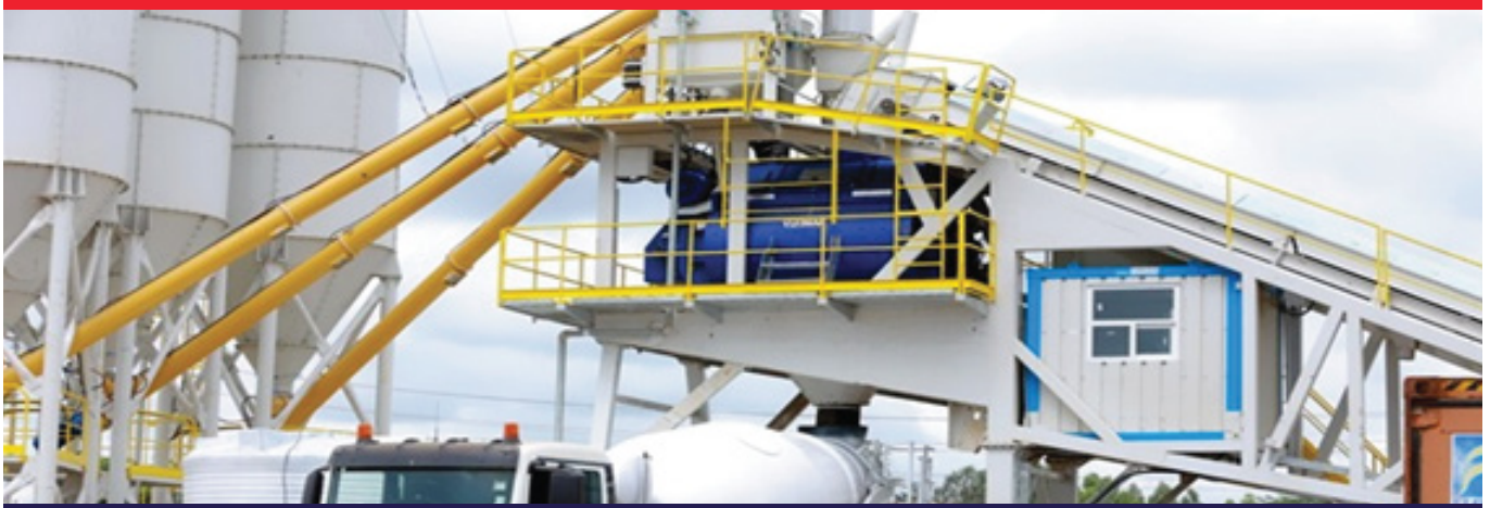
Figure 4: Ready mix concrete (RMC) manufacturing process
